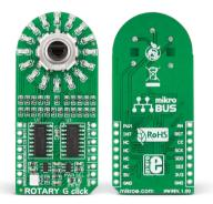
Rotary G click<sup>™</sup> carries a **15-pulse incremen**tal rotary encoder with detents, surrounded by a ring of 16 green LEDs. It communicates with the target board through mikroBUS™ SPI lines [CS, SCK, MISO, MOSI], and three additional lines for outputting the Encoder info: ENCB OUT, ENCA OUT and SW (in place of the standard AN, RST and INT pins, respectively]. Rotary G click<sup>™</sup> can be used with either a 3.3V or 5V power supply.
