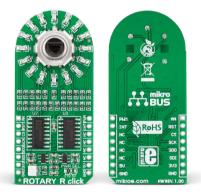
Rotary R click<sup>™</sup> carries a **15-pulse incremen**tal rotary encoder with detents, surrounded by a ring of 16 red LEDs. It communicates with the target board through mikroBUS™ SPI lines [CS, SCK, MISO, MOSI], and three additional lines for outputting the Encoder info: ENCB OUT, ENCA OUT and SW (in place of the standard AN, RST and INT pins, respectively]. Rotary R click<sup>™</sup> can be used with either a 3.3V or 5V power supply.
