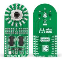
Rotary B click<sup>™</sup> carries a **15-pulse incremen**tal rotary encoder with detents, surrounded by a ring of 16 blue LEDs. It communicates with the target board through mikroBUS™ SPI lines [CS, SCK, MISO, MOSI], and three additional lines for outputting the Encoder info: ENCB OUT, ENCA OUT and SW (in place of the standard AN, RST and INT pins, respectively]. Rotary B click<sup>™</sup> can be used with either a 3.3V or 5V power supply.
