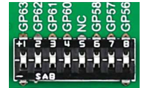
Figure 6-3: Tri-state DIP switch on PORT00-07
