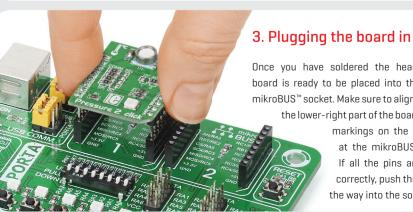
Once you have soldered the headers your board is ready to be placed into the desired mikroBUS<sup>™</sup> socket. Make sure to align the cut in the lower-right part of the board with the markings on the silkscreen at the mikroBUS<sup>™</sup> socket. If all the pins are aligned correctly, push the board all the way into the socket.
