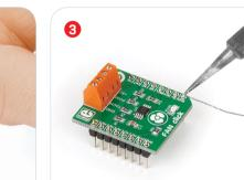
Turn the board upward again. Make sure to align the headers so that they are perpendicular to the board, then solder the
