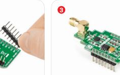
Turn the board upside down so that the bottom side is facing you upwards. Place shorter pins of the header into the pins carefully.
