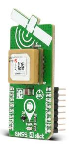
**GNSS 4 click** carries SAM-M8Q patch antenna module from u-blox. The click is designed to run on a 3.3V power supply. It communicates with the target microcontroller over I2C or UART interface.
