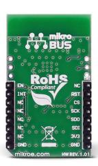
WiFi 7 click carries the ATWINC1510-MR210PB IEEE 802.11 b/g/n module, specifically optimized for low-power IoT applications. The click is designed to run on a 3.3V power supply. It communicates with the target microcontroller over SPI interface, with additional functionality provided by the following pins on the mikroBUS™ line: PWM, INT, RST.
