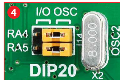
Figure 4-9: RA4 and RA5 connected to X2 quartz-crystal
