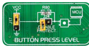
Figure 10-5: Button press level jumper (J17)
