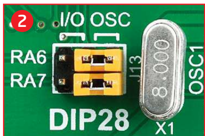
Figure 4-7: RA6 and RA7 connected to X1 quartz-crystal
