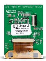
The **240x320px** screen is driven by an **FT800** graphic controller which is supported in Visual TFT, the GUI design tool for rapid development of user interfaces.
