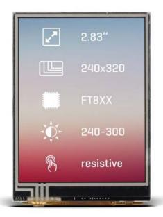
The **240x320px** screen is driven by an **FT800** graphic controller which is supported in <u>Visual</u> TFT, the GUI design tool for rapid development of user interfaces.
