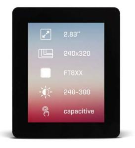
The **240x320px** screen is driven by an **FT801** graphic controller which is supported in Visual TFT, the GUI design tool for rapid development of user interfaces.
