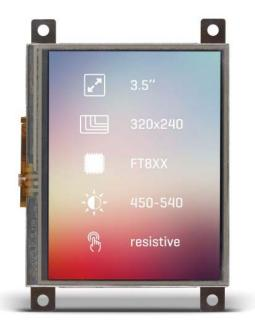
The **320x240px** screen is driven by an **FT800** graphic controller which is supported in <u>Visual</u> <u>TFT</u>, the GUI design tool for rapid development of user interfaces.
