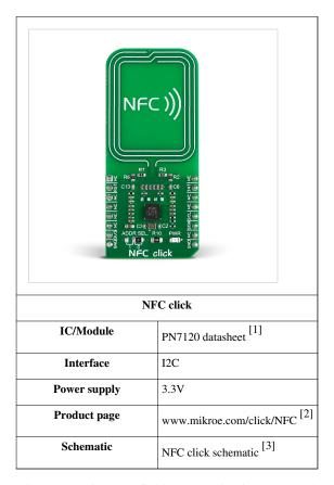
NFC click is a an add-on board with a versatile near field communications controller from NXP — the PN7120 IC. NFC devices are used in contactless payment systems, electronic ticketing, smartcards, but also in retail and advertising — inexpensive NFC tags can be embedded into packaging labels, flyers or posters.
