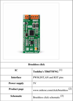
Brushless click carries Toshiba's TB6575FNG IC for driving 3-phase full-wave Brushless DC motors — which are ideal for powering flying drones. The click is able to safely drive external motors with up to 32V/2A.
