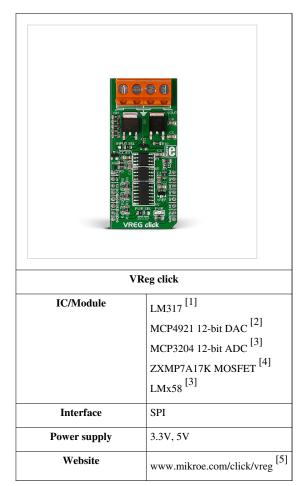
VREG click is a digitally controlled DC Voltage regulator in mikroBUS<sup>™</sup> form factor. The design is based on the well-known LM317 circuit, with the addition of a 12-bit DAC, 12-bit ADC, and an Operational Amplifier. Two pairs of screw terminals serve as inputs and outputs.
