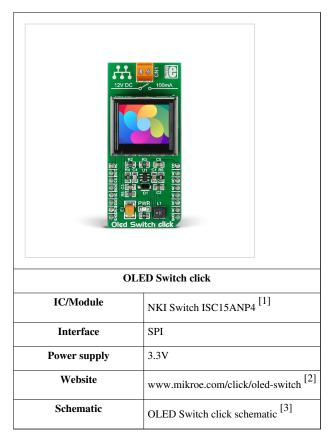
If you are building any type of human machine interface, OLED Switch click can help you keep the design simple, clear and interactive. It can be used in designing a control panel for an industrial machine... or a DIY arcade.
