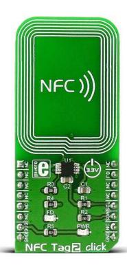
**NFC Tag 2 click** carries the NT3H1101 NTAG I2C energy harvesting NFC Forum Type 2 Tag from NXP. The click is designed to run on a 3.3V power supply only. It communicates with the target MCU over I2C interface and the INT pin (field detection) on the mikroBUS<sup>TM</sup> line.
