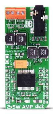
**2x5W AMP click** functions as an amplifier and features the TDA7491LP 2x5-watt dual BTL class-D audio amplifier. The click is designed to run on either 3.3V or 5V power supply. It communicates with the target MCU over the following pins on the mikroBUS<sup>TM</sup> line: AN, RST, CS, PWM, INT.
