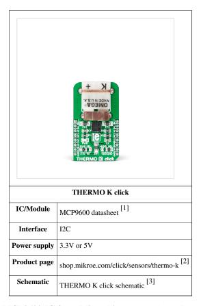
**THERMO K click** carries the **MCP9600 IC from Microchip** and and depending on the type of probe it uses, the click can measure temperatures from -200 °C to +1372 °C. THERMO K click is designed to run either on 3.3V or 5V power supply. It communicates with the target MCU through I2C interface.
