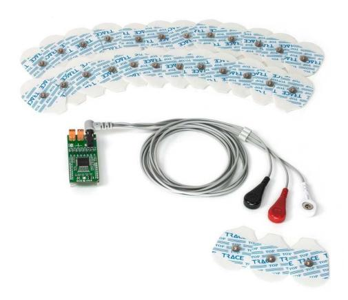
ECG 2 click bundle (the click + cable + electrodes) has what you need to start recording your ECG. Prototype your own health-tracking and fitness devices, find out how healthy your hart is or just make an LED blink in sync with your heart.
