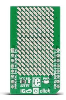
**16x9 G click** contains a **green LED matrix** and the IS31FL3731 audio modulated matrix LED driver. The dimension of the LED matrix is 16x9. Each LED can be controlled individually – both for on/off control and light intensity. The click is designed to run on either 3.3V or 5V power supply. It communicates with the target microcontroller over I2C interface and the following mikroBUS<sup>TM</sup> pins: PWM, INT, CS.
