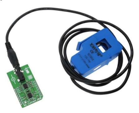
AC Current sensor is a non-invasive sensor for measuring alternating current. This split-core type of sensor can be clipped around either a live or neutral wire.
