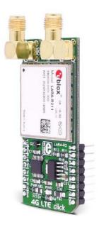
**4G LTE-E click** carries the LARA-R211 multi-mode cellular module from u-blox. The board is designed to use 5V power supply. I/O voltage levels could be 3.3V or 5V. It communicates with the target microcontroller over UART interface, with additional functionality provided by the following pins on the mikroBUS<sup>TM</sup> line: AN, RST, CS, PWM, INT.
