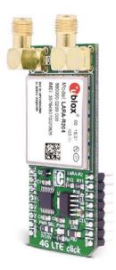
**4G LTE-NA click** carries the LARA-R204 multi-mode cellular module from u-blox. The board is designed to use 5V power supply. I/O voltage levels could be 3.3V or 5V. It communicates with the target microcontroller over UART interface, with additional functionality provided by the following pins on the mikroBUS<sup>™</sup> line: AN, RST, CS, PWM, INT
