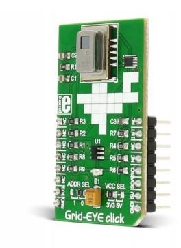
**Grid-EYE click** is a 8x8 thermal array sensor-detector that carries the AMG8853 **infrared array sensor from Panasonic**. The click is designed to run on either 3.3V or 5V power supply. It communicates with the target MCU over I2C interface.
