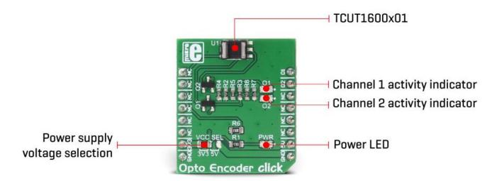
Since the signals of these two output channels are not enough to drive pins on a host MCU, the Click board™ features two additional MOSFETs. These MOSFETs are also used to drive two additional LEDs, which indicate activity of each channel. E1 and E2 pins are routed to the MOSFET gate pins, while the MOSFET drains are routed to the mikroBUS™ PWM and INT pins. These pins are pulled to a LOW logic level by the pull-down resistors, to avoid floating.
