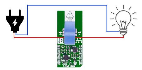
There is on board ADC to read out the analog output value of the sensor, or it can be read from the AN pin.
