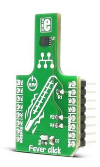
**Fever click** measures your body temperature with the accuracy of 0.1°C (37°C to 39°C). The click carries MAX30205 human body temperature sensor. Fever click is designed to work on a 3.3V power supply. It communicates with the target MCU over I2C interface.
