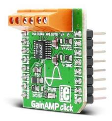
**GainAMP click** carries the LTC®6912 dual channel, low noise, digitally programmable gain amplifier (PGA). The click is designed to work on either 3.3V or 5V power supply. It communicates with the target MCU over SPI interface, with additional functionality provided by the following pins on the mikroBUS<sup>TM</sup> line: AN, RST.
