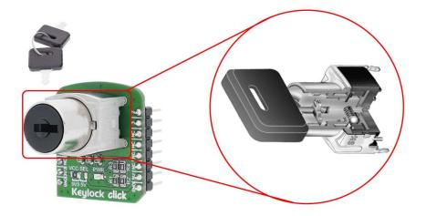
The key can be removed from the lock in any of the three positions. The package contains two keys and one protective cap.
