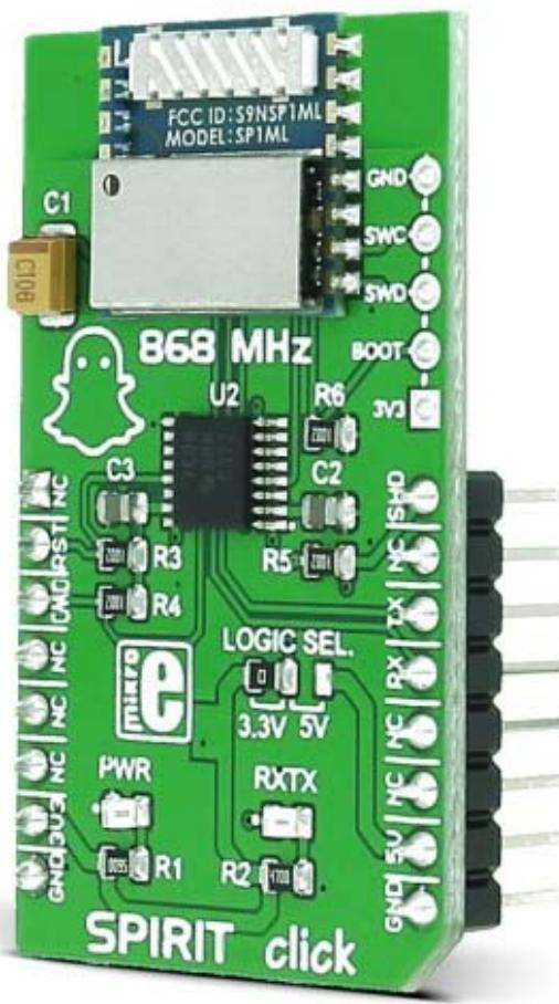
**SPIRIT click** carries the SP1ML 868MHz ultra low-power RF module. The board is designed to use 3.3V power supply and 3.3V or 5V I/O voltage levels. It communicates with the target MCU over UART interface, with additional functionality provided by the following pins on the mikroBUSTM line: PWM, RST, CS.
