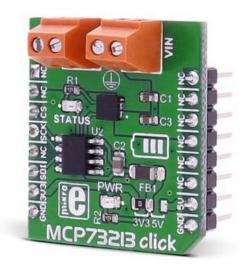
MCP73213 click carries the MCP73213 dual-cell Li-Ion/Li-Polymer battery charge management controller with input overvoltage protection from Microchip. The click is designed to run on either 3.3V or 5V power supply. It communicates with the target microcontroller over SPI.
