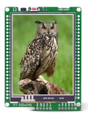
**Mikromedia for PIC18FK** is a compact smart display and development platform with the PIC18F67K40 microcontroller from Microchip. The large 320x240 TFT color display will allow you to build multimedia applications with speed and ease. You can use it for development and as a final product.
