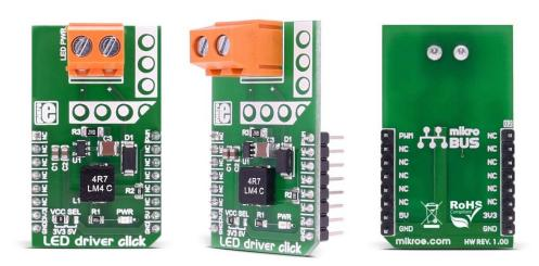
**LED driver click** carries the MCP1662 high-voltage step-up voltage driver from Microchip. The click is designed to run on either 3.3V or 5V power supply. It communicates with the target microcontroller over PWM pin on the mikroBUS™ line.
