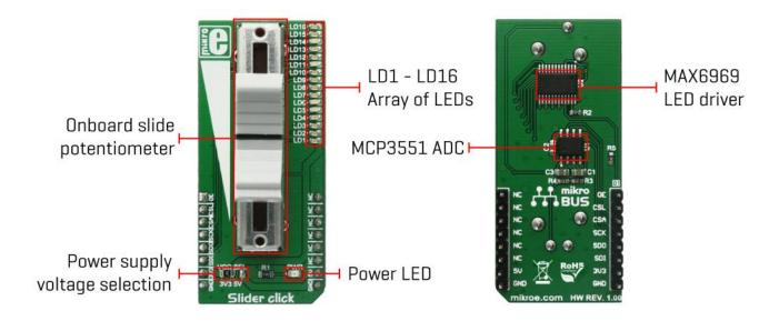
This click board<sup>TM</sup> can work with both 3.3V and 5V, depending on the used MCU capabilities. This can be done by switching the VCC SEL SMD jumper to the desired position.
