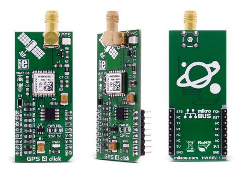
**GPS 4 click** carries the L70 compact GPS module from Quectel. The click is designed to run on either 3.3V or 5V power supply. It communicates with the target microcontroller over UART interface, with additional functionality provided by the following pins on the mikroBUS™ line: PWM, AN, RST.
