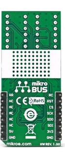
**7x10 G click** can be used for displaying letters on a display with 7x5 font resolution. It carries a matrix of 70 green LEDs driven by a pair of 8-bit serial-in, parallel-out shift registers, a Darlington Transistor array and a Johnson counter.
