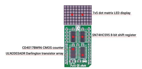
The dot matrix can also show scrolling text, thus fitting longer messages in small space. The pair of 8-bit SIPO shift registers drive the display. The current amplification necessary for driving the LEDs is performed by a Darlington Transistor array while a Johnson counter performs the necessary LED multiplex.
