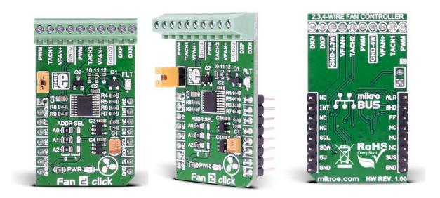
**Fan 2 click** carries the MAX31760 precision fan-speed controller. It can measure temperature and adjust the fan speed to keep the temperature at the same level. Fan 2 click can also control two fans at the same time.
