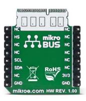
Add memory to your project with **EERAM 3.3V click**. It carries the <u>47L16</u> EERAM, a 16Kbit SRAM with **EEPROM Backup** from Microchip. The click is designed to run on a 3.3V power supply. It communicates with the target microcontroller over I2C interface, with additional functionality provided by the INT pin on the mikroBUS<sup>TM</sup> line.
