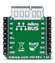
Add memory to your project with **EERAM 5V click**. It carries the 47C16 EERAM, a 16Kbit SRAM with EEPROM Backup from Microchip. The click is designed to run on a 5V power supply. It communicates with the target microcontroller over I2C interface, with additional functionality provided by the INT pin on the mikroBUS<sup>TM</sup> line.
