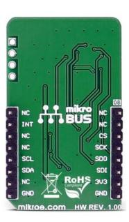
**LSM6DSL click** measures linear and angular velocity with six degrees of freedom. It carries the LSM6DSL high-performance 3-axis digital accelerometer and 3-axis digital gyroscope. The click is designed to run on a 3.3V power supply. LSM6DSL click communicates with the target microcontroller over SPI or I2C interface, with additional functionality provided by the INT pin on the mikroBUS<sup>TM</sup> line.
