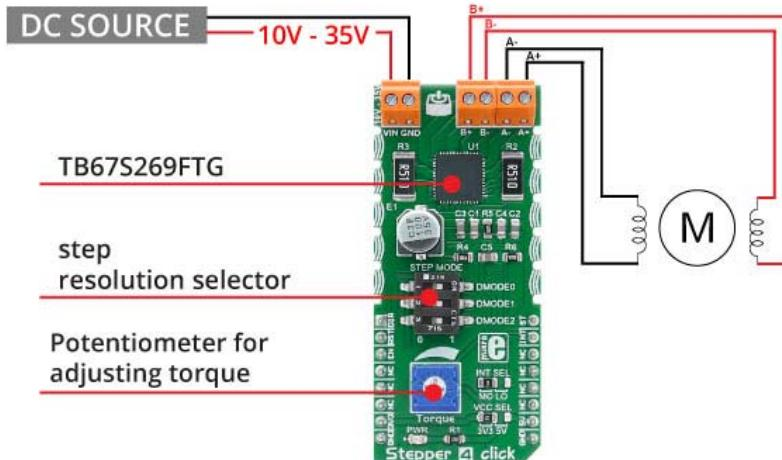
The other four connectors are used for connecting the stepper motor to the click. After a motor is connected, it can be controlled by the MCU through the Stepper 4 click.
