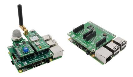
Picture on the right shows Pi 3 click shield connected to the Raspberry Pi® 3 model B, picture on the left shows the connected shield along with two click boards<sup>TM</sup>: Ozone 2 and GNSS 5 click.
