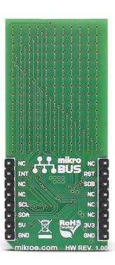
16x12 G click carries a 16x12 LED display and the IS31FL3733 matrix driver. The click is designed to run on either 3.3V or 5V power supply. It communicates with the target microcontroller over I2C interface, and the following pins on the mikroBUS™ line: INT, RST, CS.
