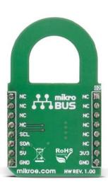
**Secure 3 click** carries the ATSHA204A, a cryptographic coprocessor with secure hardware-based key storage from Microchip. The click is designed to run on either 3.3V or 5V power supply. Secure 3 click communicates with the target microcontroller over an I2C interface.
