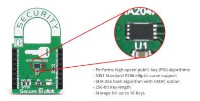
The ATSHA204A device includes an Electrically Erasable Programmable Read-Only Memory (EEPROM) array that can be used for key storage, miscellaneous read/write data, read-only, secret data, consumption logging, and security configuration. Access to the various sections of memory can be restricted in a variety of ways, and the configuration can then be locked to prevent changes.
