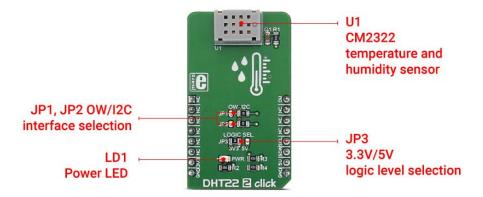
Typical temperature accuracy is  $\pm 0.3$  °C, while relative humidity accuracy is 2% RH, with the resolution of 0.1 for both measured properties.
