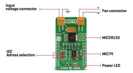
Fan 3 click can be used on several different I2C addresses, selectable by the ADD SEL jumpers. Those jumpers are used to directly set A0 to A2 address select pins of the MIC74. By default, all address pins are grounded, which sets the slave I2C address to 0x20h.
