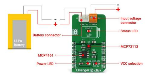
If a Li-Ion battery is discharged to below 3V, it has to be pre-charged with around 10% of the full charge current. This means that the charging current, in this case, will be 10% of the fast charging current set by the MCP4161 digital potentiometer.
